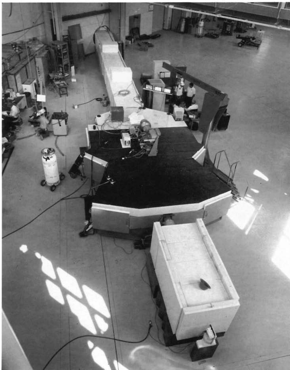
The Neutron Powder Diffractometer was the first instrument to be installed in the new addition to the experiment hall. The d -spacing resolution of this diffractometer is better than that of any other instrument of its type in the United States.
